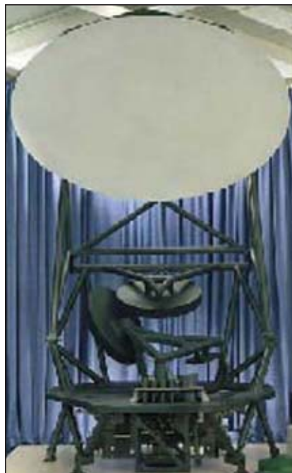
▲ Fig.11 Full scale model of the CMIS instrument (courtesy of NOAA). 13
