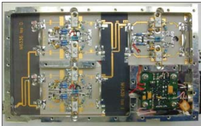
▲ Fig. 2 35 W output rank power amplifier module construction.
