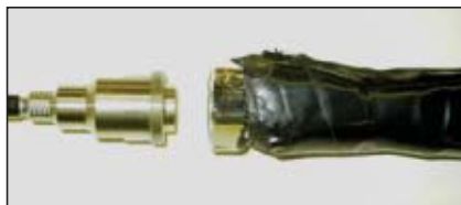
▲ Fig. 2 Connection between an analyzer test cable and a site jumper cable.
