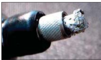
▲ Fig. 4 Failed cable attachment.
