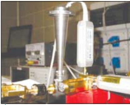
▲ Fig. 9 OMT test setup.
