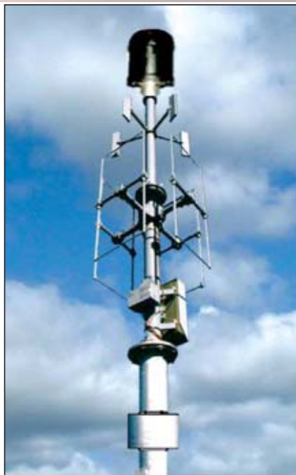
▲ Fig. 1 Combined antenna array for radar and COMMS signals.
