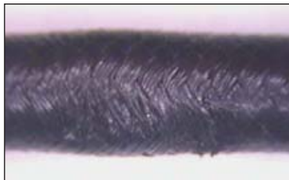
▲ Fig. 3 Dented coaxial cable.
