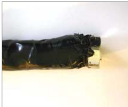
Fig. 1 Actual cell site disconnected jumper cable. ▼
